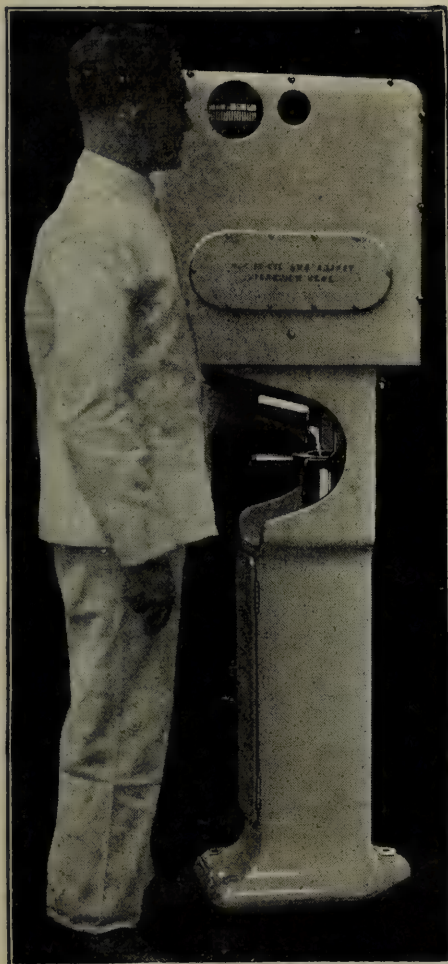
Fig. 107. Adjusting the Overrun Cup for any Composition of Mix. Remove the Cup of Mix from the Scale, and Place the Slotted Base on the Metal Cleat Under Weighing Frame.
